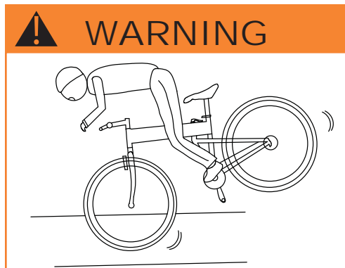
Fig. 6: Using too much braking pressure on the front wheel can cause you to lose control.
