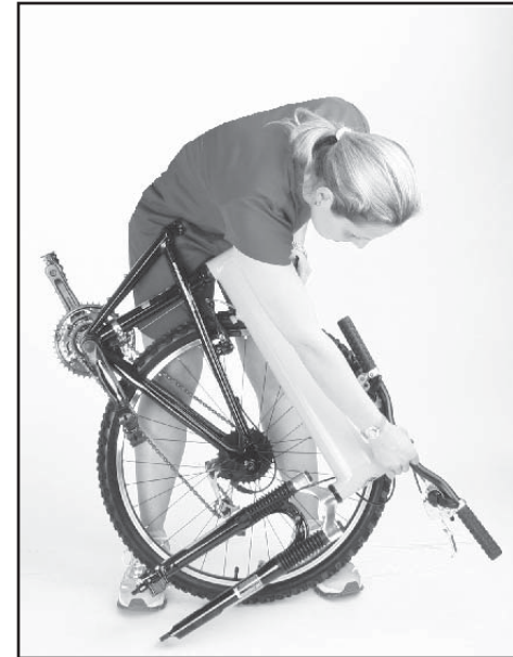
Fig. 13: Folding the Montague Bike
