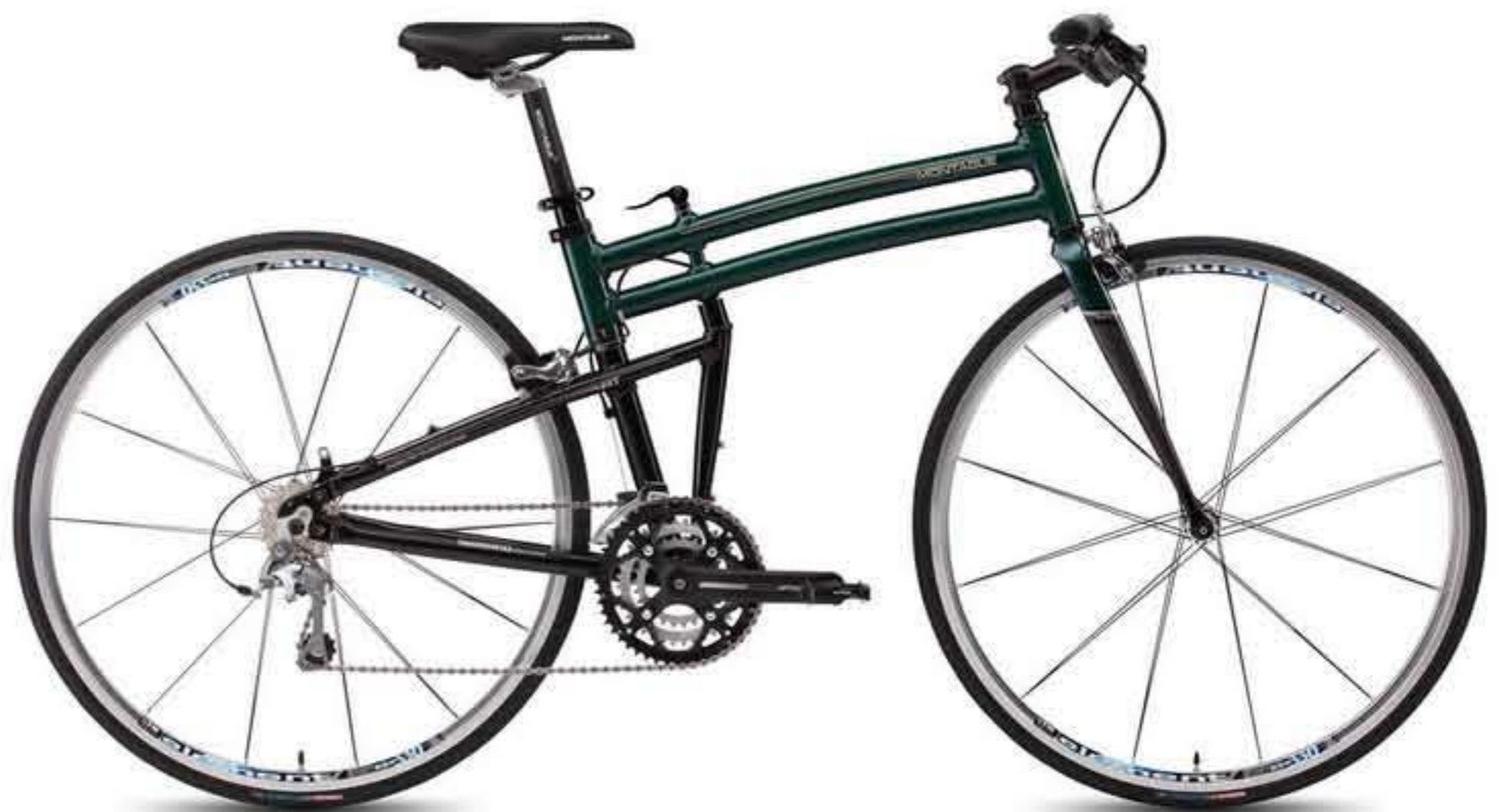
In 2010, Montague debuted a full-size foldable bike designed for pavement riding, with frames of 19" or 21" for shorter or taller riders, 700c wheel size, and 30 speeds.
