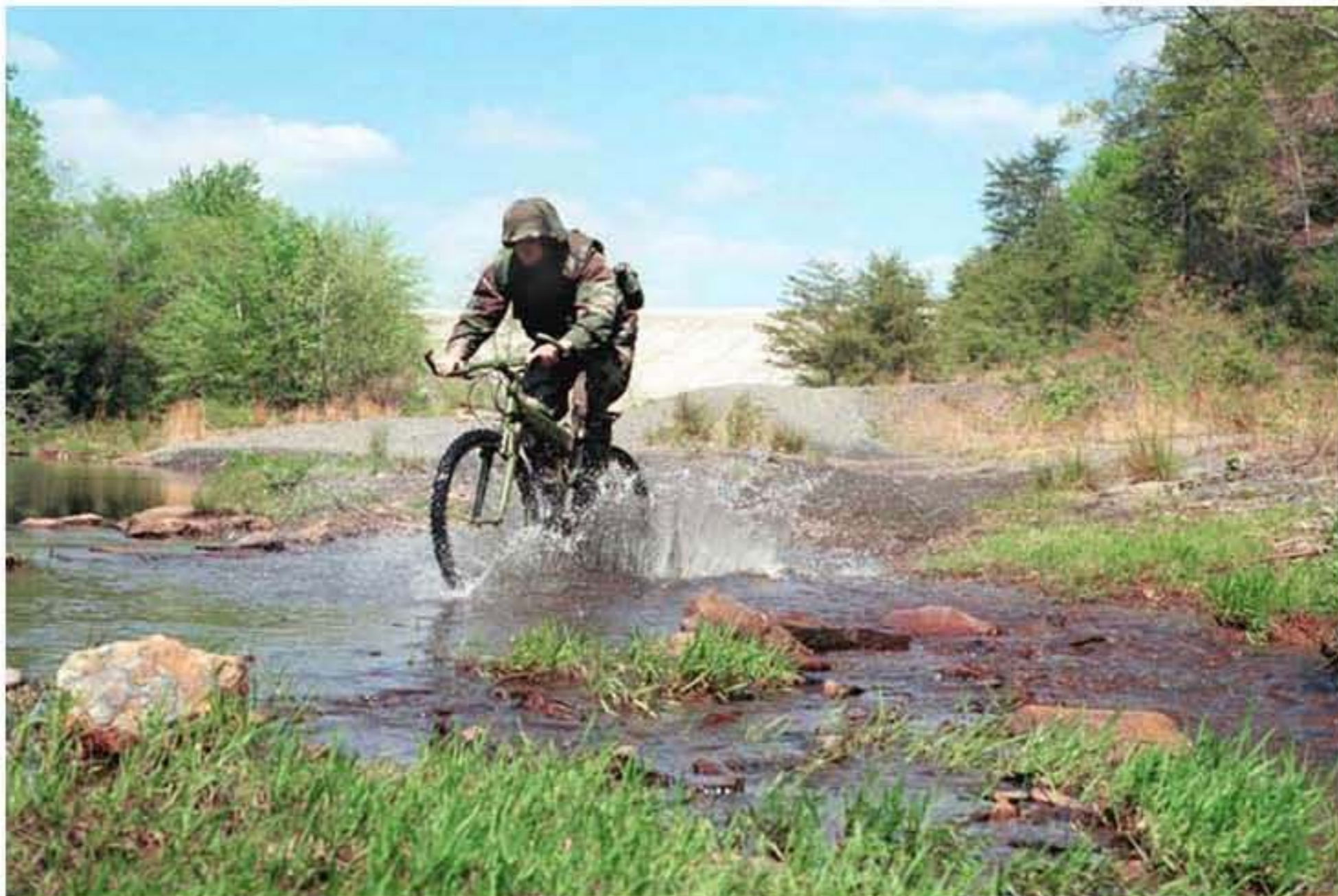
Soldiers can get around on a bike rather than on foot. Paratrooper bikes for the military were made with airless tires to avoid flats and no chrome that could reflect.
