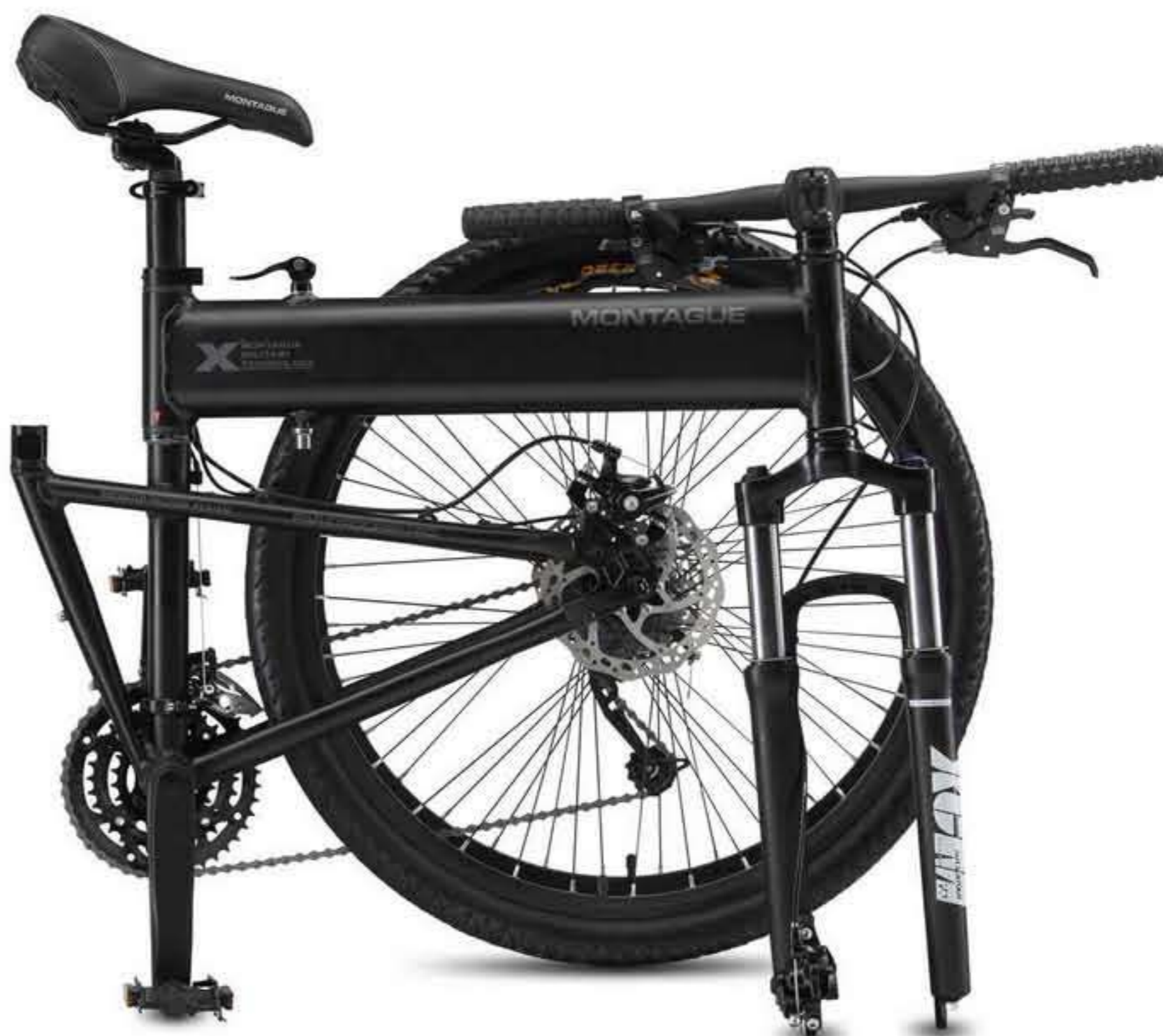
Montague Paratrooper Pro mountain bike folds to 36”x28”x12”, and weighs approximately 29 lbs.
