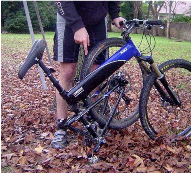
Step 3: Twist the rear triangle around
