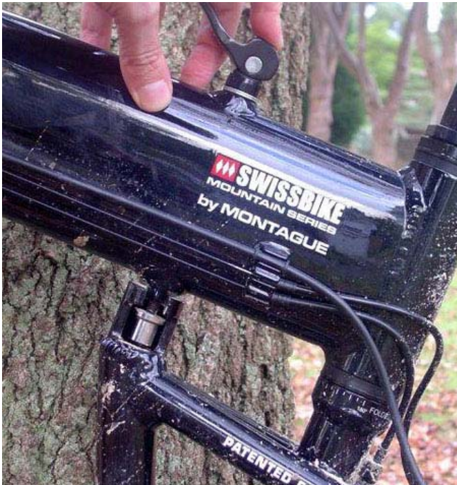
Step 2: Release the lever that fastens the rear triangle
