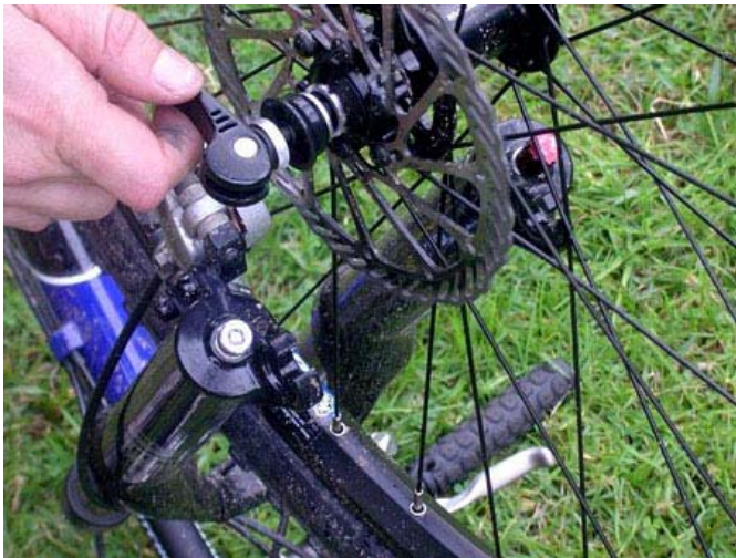
Step 4: Detail - removing the front wheel - once handed with the springed skewer
